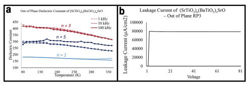
Figure 5: (a) For all of the samples measured, there is no clear peak, and therefore, ferroelectric transition indicated. Compared to in-plane, out-of-plane dielectric constants are much lower. (b) This measurement shows that for even voltages as low as perhaps 5V, the leakage current measured is extremely high.
