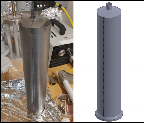
Figure 2: Old vs. new differential pumping sleeve.
