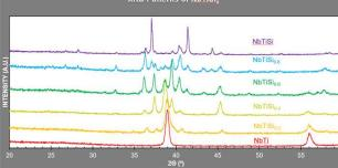
As more silicon is added to the pure NbTi phase, binary Nb<sub>5</sub>Si<sub>3</sub>, Nb<sub>3</sub>Si, and TiSi<sub>2</sub> phases start to become the majority phases in the diffraction pattern
