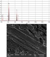
A scanning electron microscope will be used to verify the chemical composition of the alloy samples. Nanoindentation will also be used to test the mechanical strength of the materials post box furnace oxidation.
