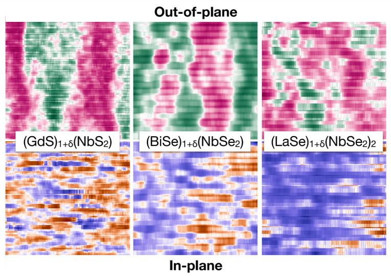
Similar large-scale coherent out-of-plane distortions were found in the Bi and La compounds. In contrast, the scale and frequency of coherent in-plane distortions differs between the compounds.
