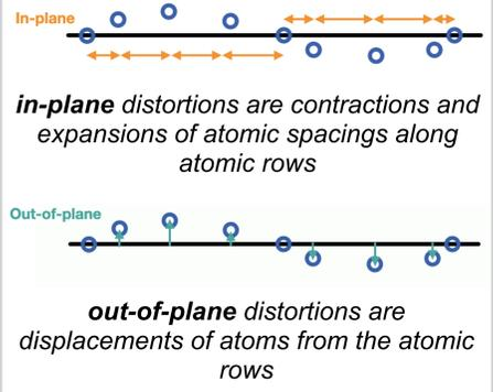
Quantifying these picometer-scale structural distortions required the development of a careful analytical framework to define and create an appropriate reference.
