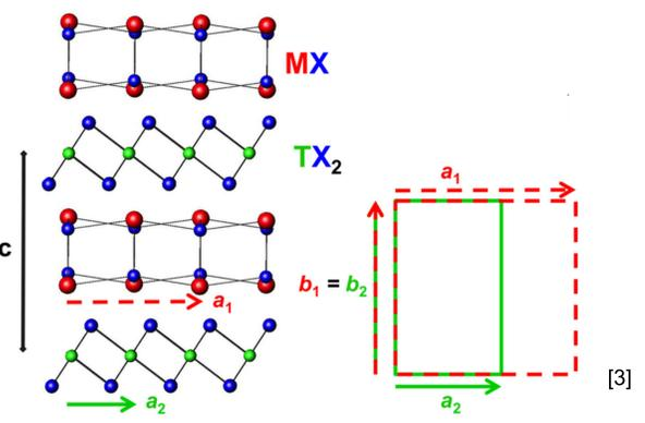
The primary objective of this work was to understand and quantify the differing structural responses of three misfit compounds—(GdS)<sub>1+δ</sub>(NbS<sub>2</sub>), (BiSe)<sub>1+δ</sub>(NbSe<sub>2</sub>), and (LaSe)<sub>1+δ</sub>(NbSe<sub>2</sub>)<sub>2</sub>—and the distinct manner in which they accommodate the misfit in lattice parameters.
