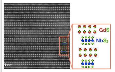
Three misfit compounds were imaged on a Thermo Fisher Scientific Spectra 300 X-CFEG STEM to probe in-plane and out-of-plane distortions.
