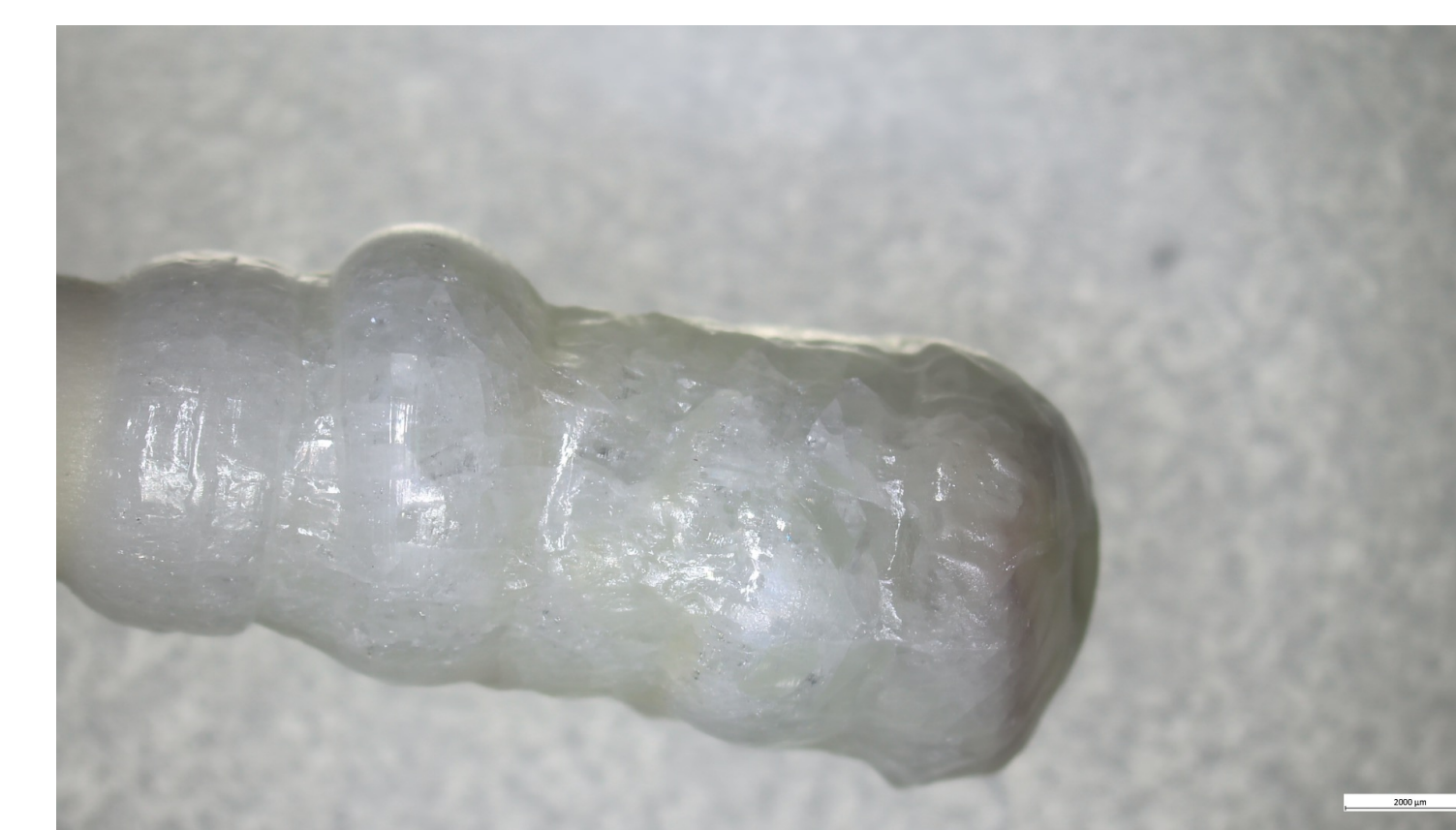
Figure 7. First floating zone single crystal of \text{CaWO}_4
