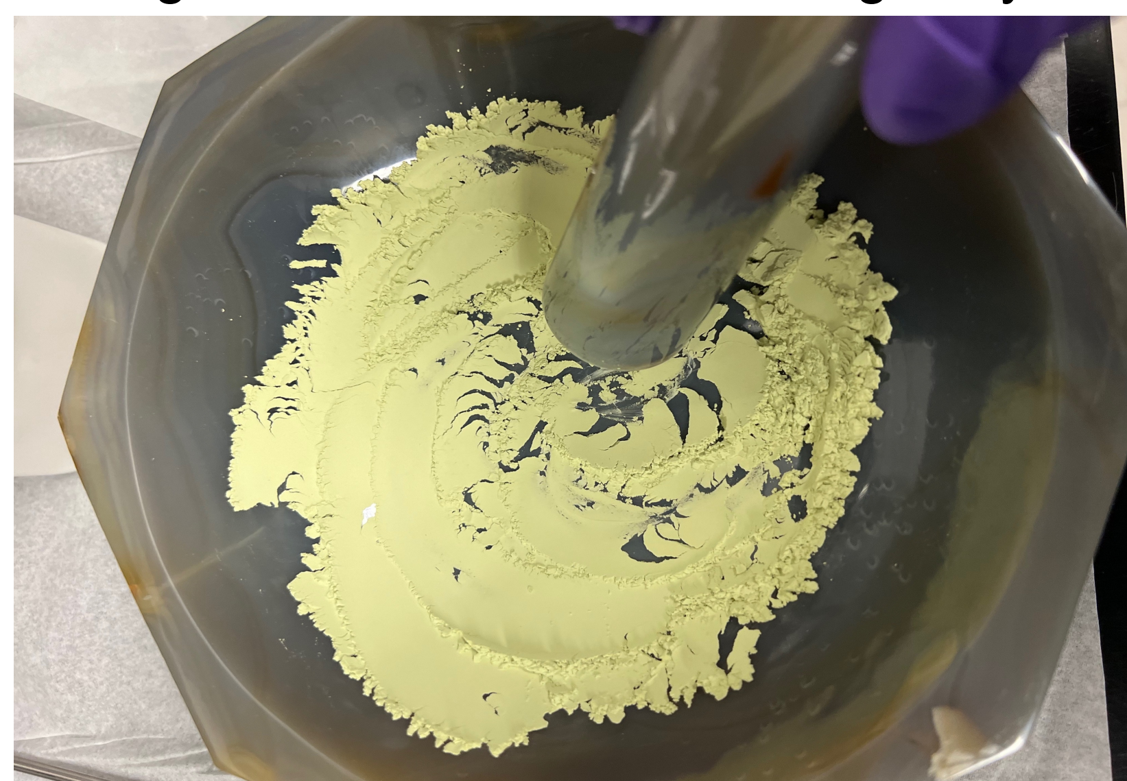
Figure 3. \text{CaCO}_3 + \text{WO}_3 \rightarrow \text{CaWO}_4
