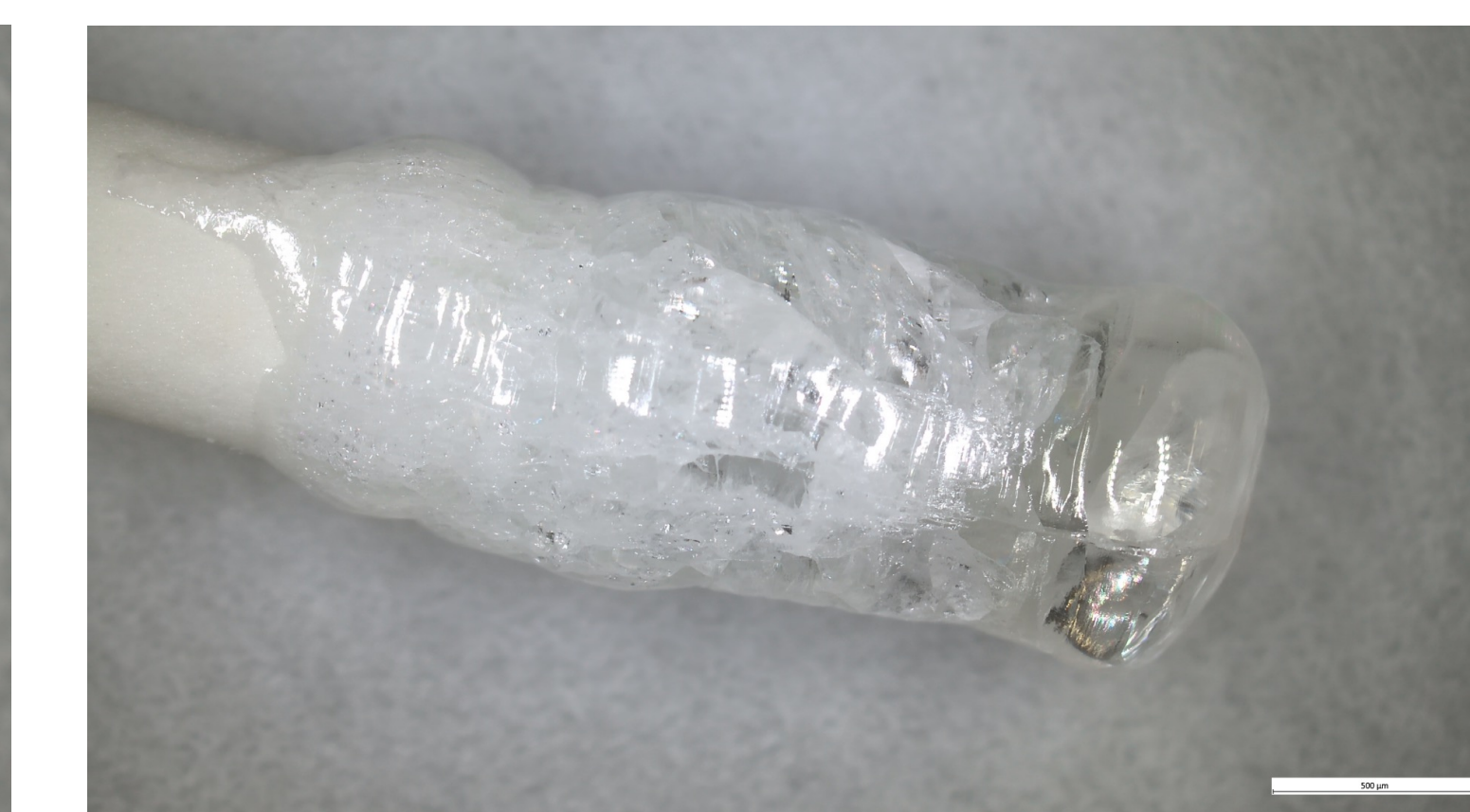
Figure 8. Second floating zone single crystal of \text{CaWO}_4
