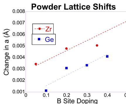
Determination of dopant level within a given sample was determined via the lattice parameter shift. The addition of metallic ions of varying size on the B site of the perovskite will cause small, yet determinable changes in the lattice parameters, despite the identity of the compound remaining the same when evaluated via powder XRD.
