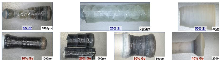
With increasing dopant percentage, the crystals became lighter and more opaque, and they had less stable molten zones in the growth process. In addition, the more dopant that was placed in the sample, the more sensitive that sample was to air.
