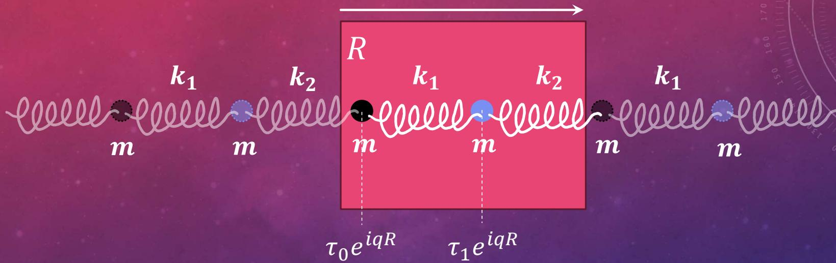
$$-D(q) = e^{-iq(-R_1)} \begin{pmatrix} 0 & 0 \\ k_2 & 0 \end{pmatrix} + \begin{pmatrix} -(k_1 + k_2) & k_1 \\ k_1 & -(k_1 + k_2) \end{pmatrix} + e^{-iq(+R_1)} \begin{pmatrix} 0 & k_2 \\ 0 & 0 \end{pmatrix}$$
