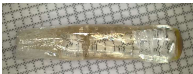
Figure 3. Single crystal of Yb:YVO_4 synthesized via laser-diode floating zone. Scale = 1mm.
