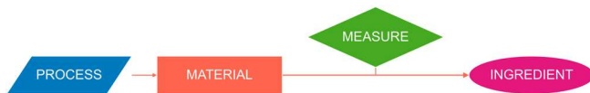
Figure 4. A diagram of the typical nodes used in a typical GEMD data model. Each node contains information pertaining to relevant attributes and is connected by directed edges.
