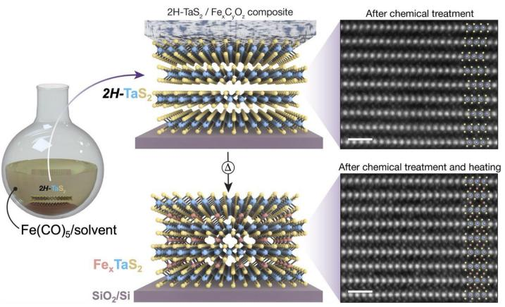
(Left) Schematic of depositing Fe precursors onto 2H-TaS<sub>2</sub> crystals on SiO<sub>2</sub>/Si support followed by vacuum annealing to yield Fe-intercalated 2H-TaS<sub>2</sub> (Fe<sub>x</sub>TaS<sub>2</sub>). (**Right**) Atomic resolution electron microscopy after chemical treatment (**top**) plus annealing at 350 °C for 30 minutes (**bottom**). Scale bars 1 nm.
