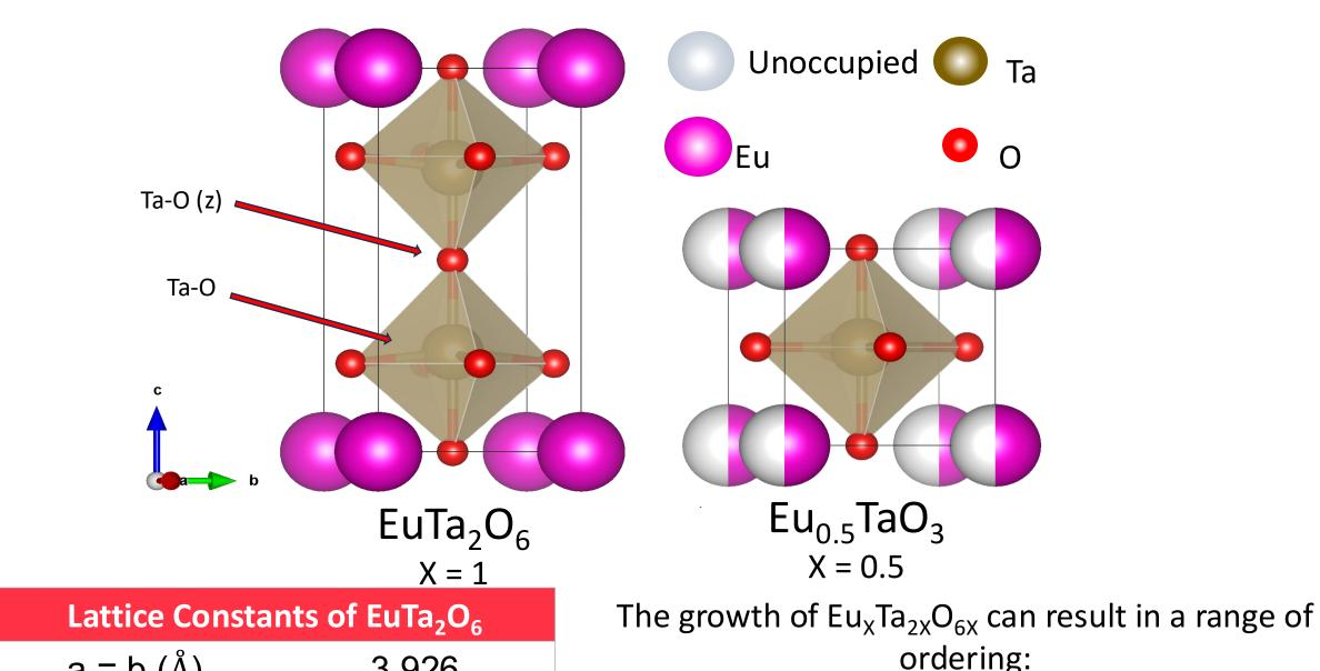
a = b (Å)3.926 X = 1 being the most ordered structure with 7.929 c (Å)
