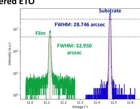
XRD scans (left) of disordered and ordered ETO with corresponding rocking curves (right) that show close full-width half max values of the substrate and film
