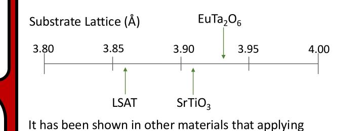
compressive strain on film by substrate can improve ordering of your crystal.
