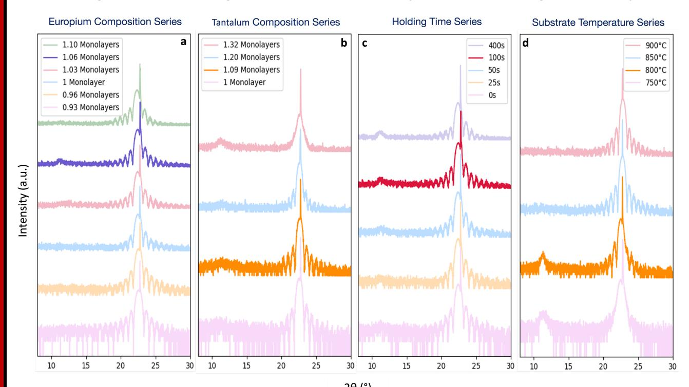
X-ray Diffraction scan series depict variation of growth parameters to determine optimal conditions for higher ordering in ETO. a) Europium composition series b) Tantalum composition series c) Holding time between unit cells series d) Substrate Temperature series
