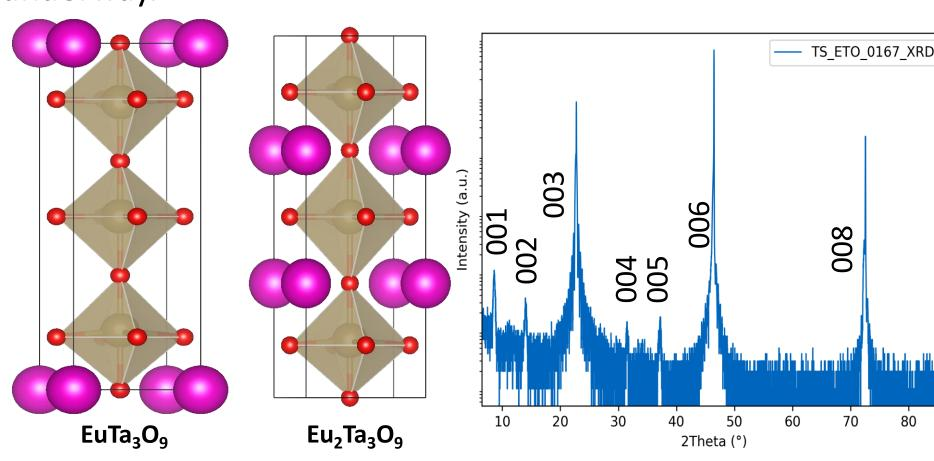
Potential structures of ETO with an additional *B*-site layer.
