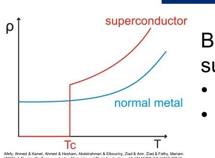
Below a critical temperature (T<sub>C</sub>), superconductors:
