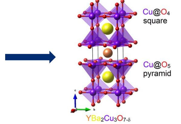
Cuprate superconductors have the highest T<sub>C</sub> at ambient pressure. Properties of the copper oxide (CuO<sub>2</sub>) layers are theorized to be the mechanisms for superconductivity.
