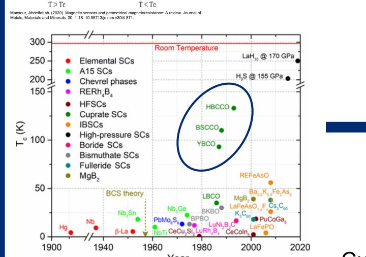
Applications are limited due to low critical temperatures, requiring liquid He or liquid N to cool to superconducting state.
